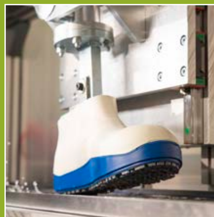
SLIP RESISTANCE TEST
